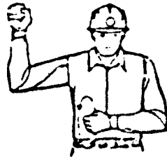
FOR MOBILE CRANES LOCK THE CRAWLER BELT ON SIDE INDICATED BY RAISED FIST TRAVEL OTHER CRAWLER BELT IN DIRECTION INDICATED BY REVOLVING FIST
